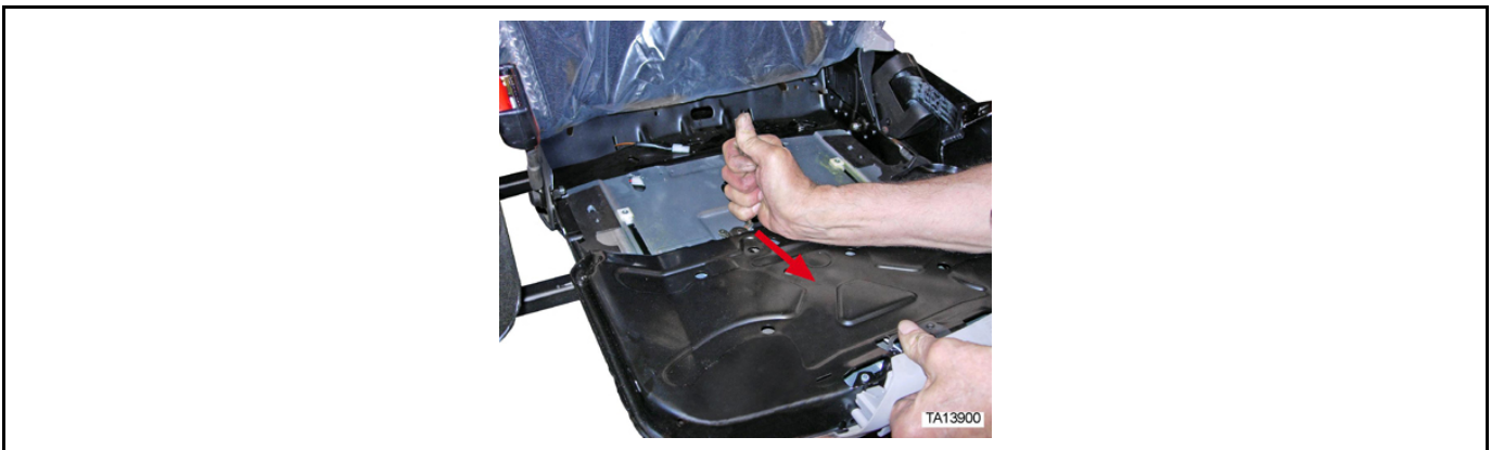
Figure 25: Seat cushion slide mechanism moved past stop to align plastic tabs with square slots in seat cushion slide mechanism
