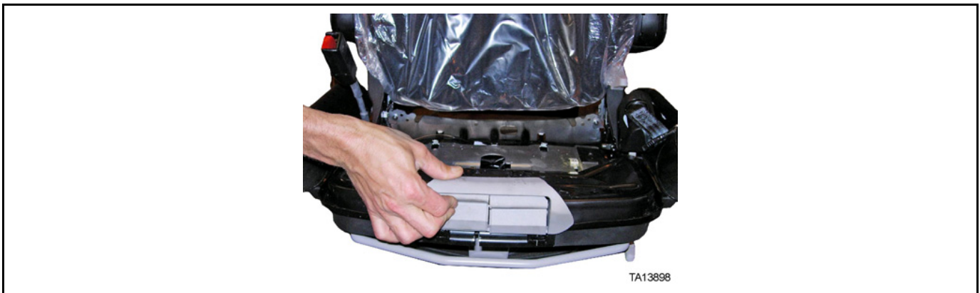
Figure 23: Seat cushion slide mechanism release lever (Compress and move seat cushion slide mechanism forward to stop)
