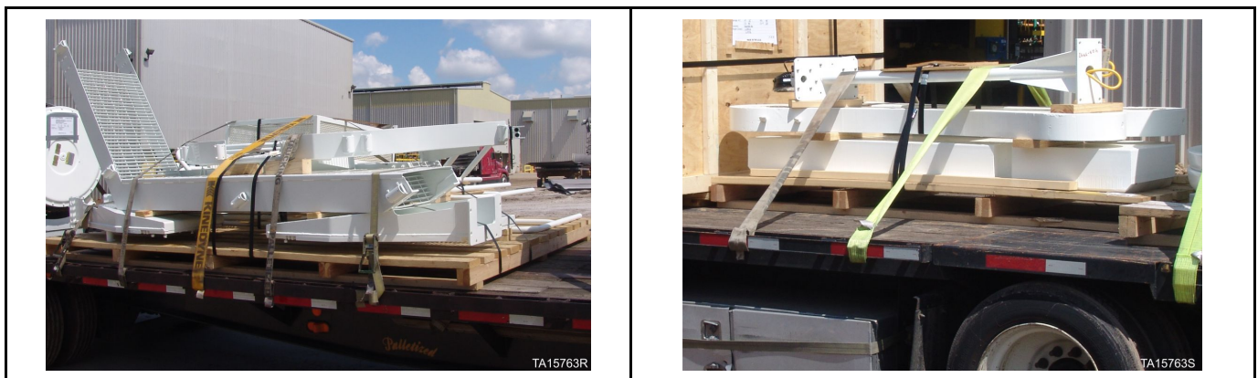
Figure 108: Typical tie down locations on miscellaneous steel structures
