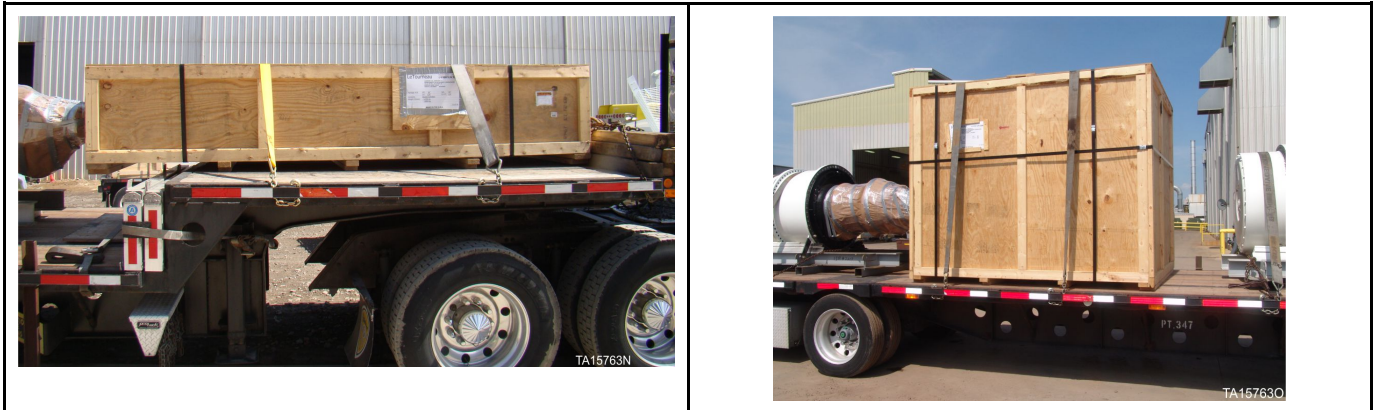
Figure 109: Typical tie down locations on crates containing miscellaneous parts such as cab and light bar
